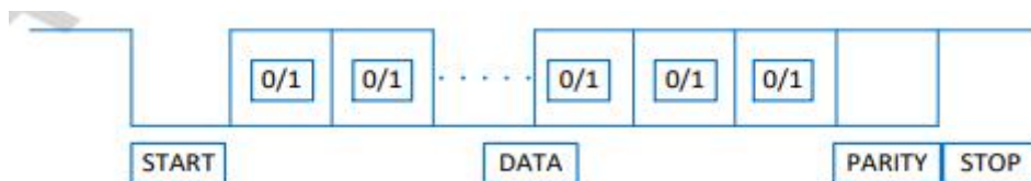
Figure 12 LPUART data transmission format
